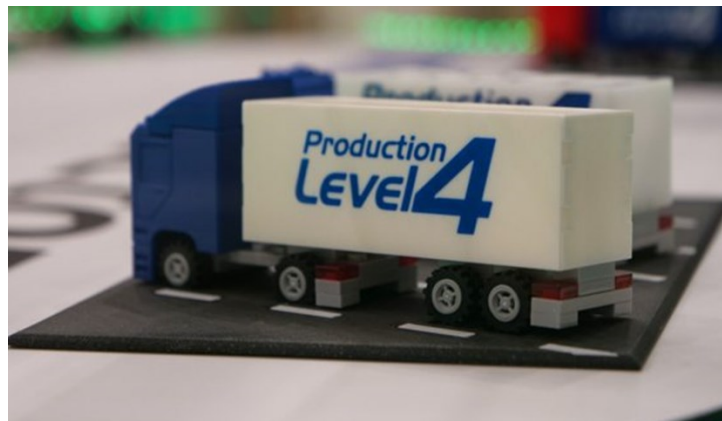
Figure 33: Sample product of SmartFactory KL is a model-sized truck where the colors, geometries, materials and manufacturing processes can be configured individually.
